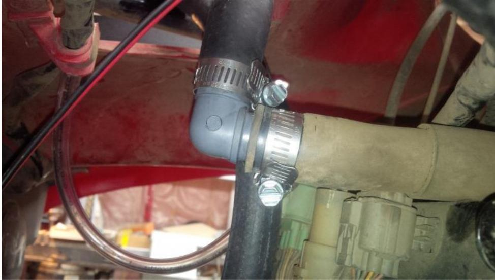
**-Connect the supplied 1/4" Clear hose to the factory overflow hose using the supplied 1/4" Brass hose barb, then put the other end of the clear hose on the overflow nipple at the fill neck of the radiator.**
