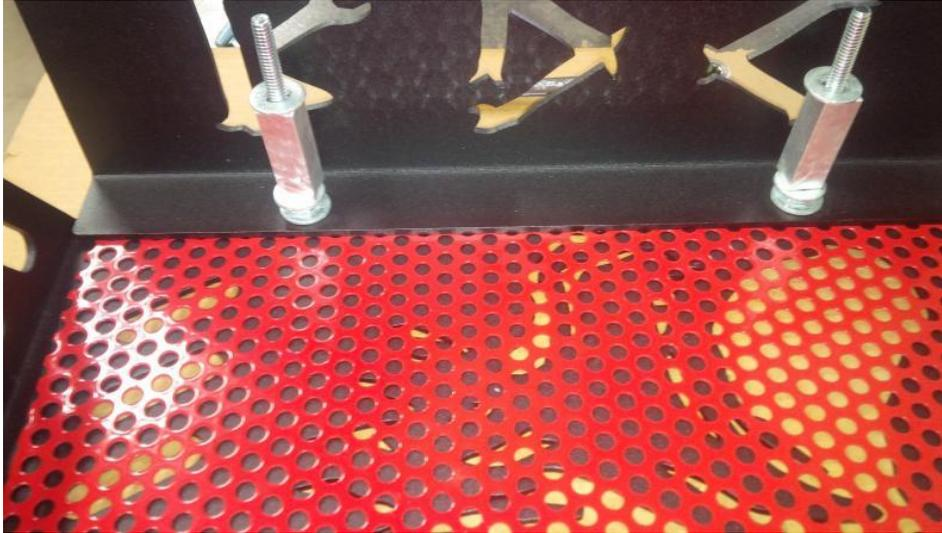
**-Remove the factory threaded clips from the radiator that were used for bolting the fan to the radiator.**
