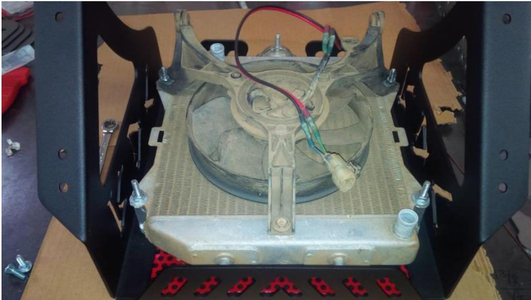
**Place the radiator bracket with rad kit and fan attached, onto the front rack and bolt in place with the 3/4" U-bolts, flat washers and 1/4" NYLOCK nuts.**
