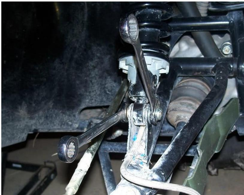
Slide a 3/8" x 2" bolt through one of the lift plates pointing towards the back of the machine, through hole "A", then slide the bolt through the stock shock mounting bracket, and through the aluminum spacer provided. Place the other lift plate using the same hole "A" on the threads of that bolt and put a nut on the bolt, **BUT ONLY PUT IT ON A COUPLE OF THREADS!**
