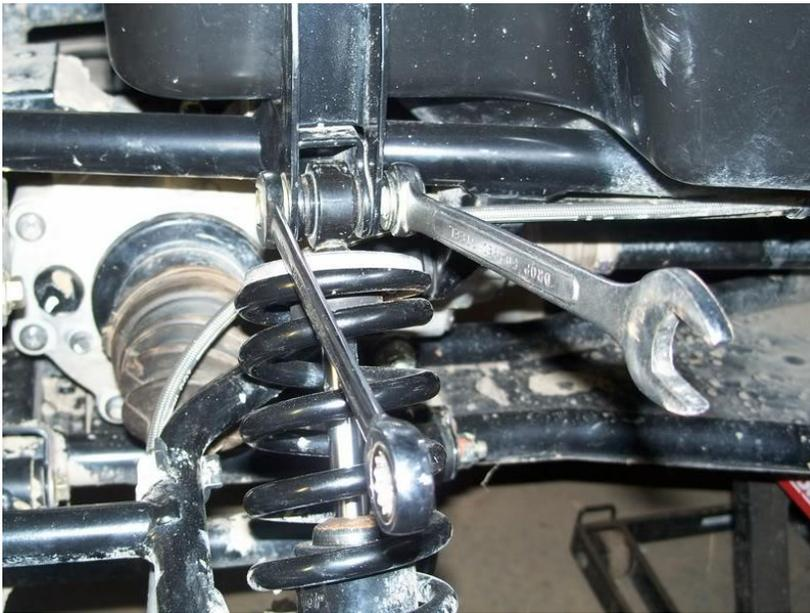
Loosen the a-arm bolt pictured below, loosen it enough that the nut almost comes off the bolt, but not quite all the way, then push it towards the back of the machine so the head of the bolt is pushed towards the rear of the machine leaving a space for one of the brackets.
