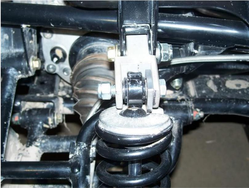
Its kind of tricky, but you now need to get the open end of the long curved bracket to hook over the a-arm bolt you loosened, then have the square end of that bracket line up with the hole in the lift block inside the channel on the block, but on the forward side of that channel or machined slot.
