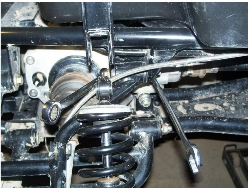
Now the lift block and bracket need to be installed in the stock shock mounting hole, make sure the offset side of the rear block is towards the back of the machine as pictured below...
