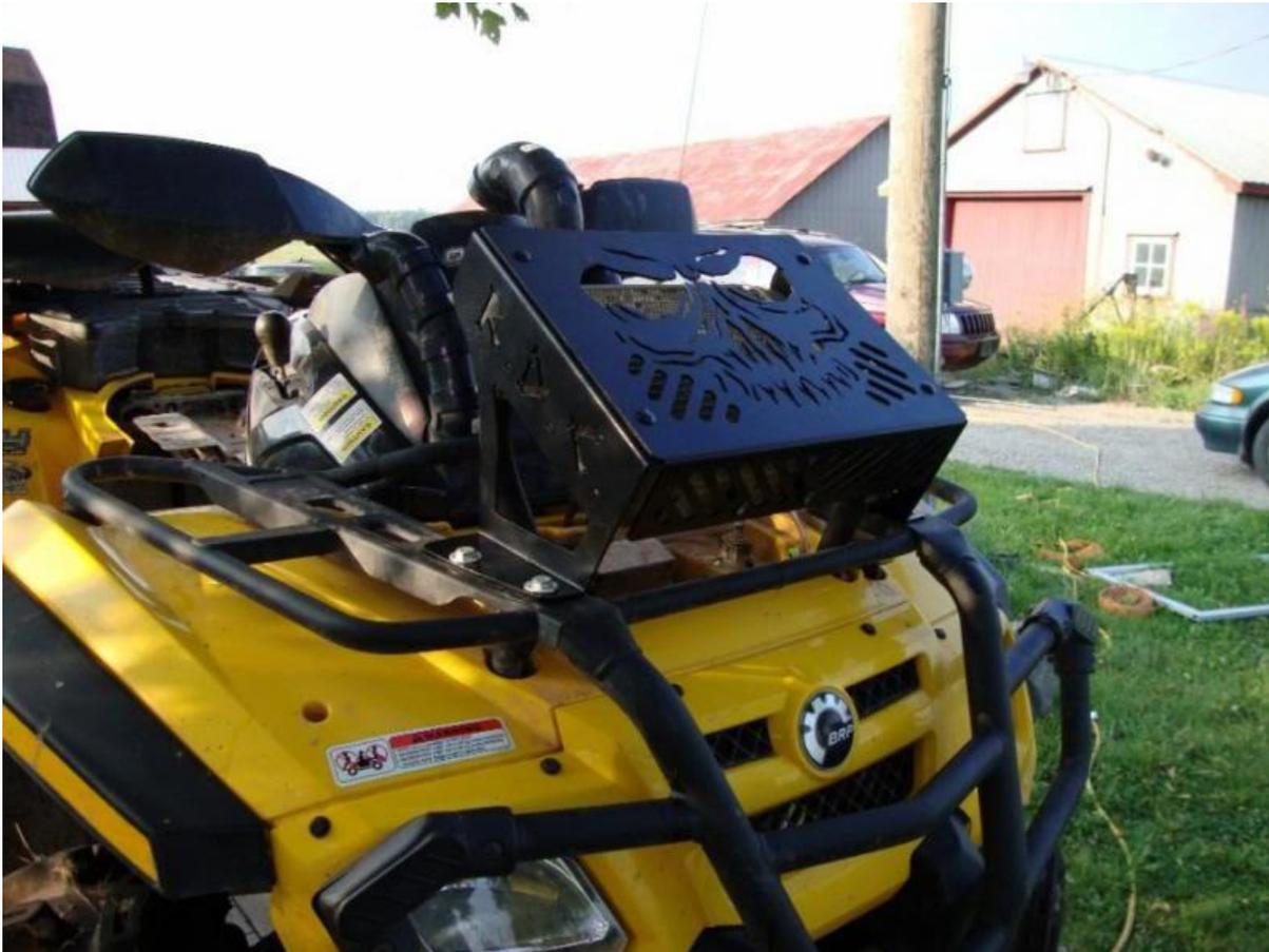
You will now need to pick the perfect spot to drill your holes for the radiator hoses, just make sure before you drill them that they will not interfere with anything you cant drill or cut through under the factory rack. Mark your hole locations and remove the bracket and cut/drill all of your holes. Some people prefer to just remove the stock plastic center cover all together.
