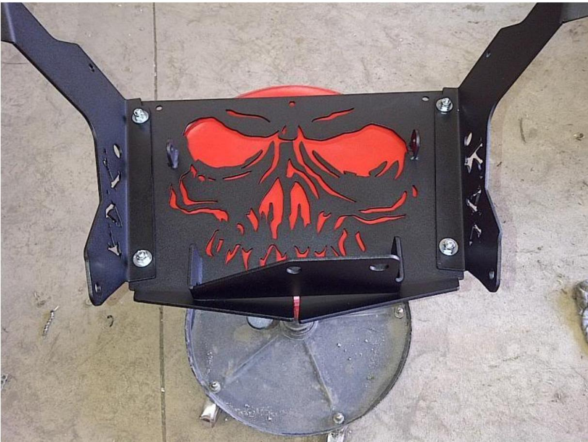
**Install hardware onto the mounting base plates and bolt them to the front rack as pictured below, it is usually best to leave them slightly loose until **EVERYTHING** is installed to make sure everything lines up perfectly,**
