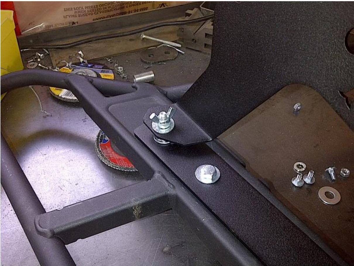
Place your radiator into the new bracket and bolt it in with the 2 factory bolts that were used to hold it in the factory location.
