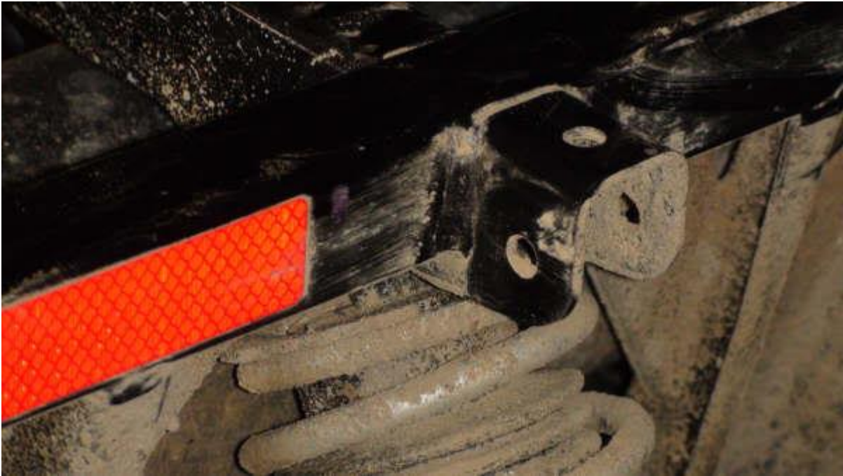
Lift Block installed on rear left side,
