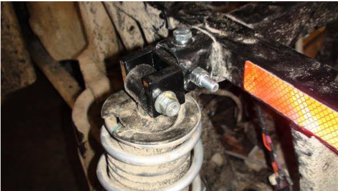
Shock mounted in lift block, rear left side,
