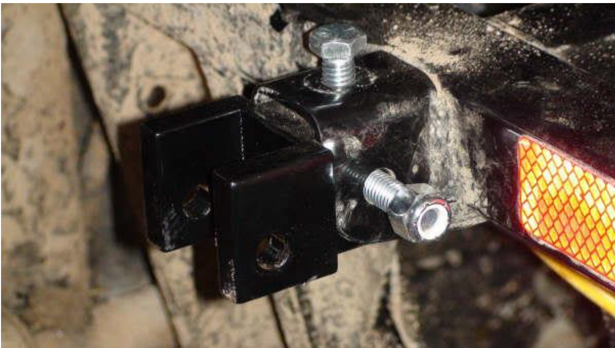
Lift Block installed on rear left side,
