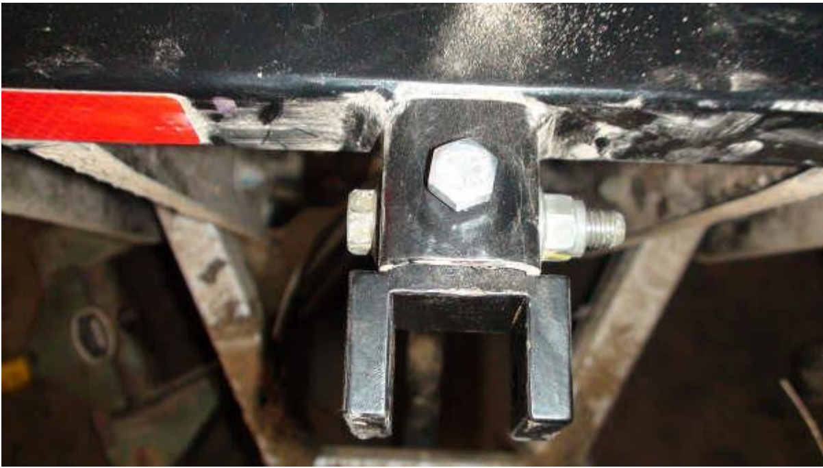
Shock mounted in lift block, rear left side,
