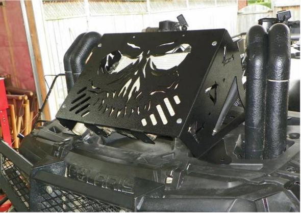
You will now need to pick the perfect spot to drill your holes for the radiator hoses, just make sure before you drill them that they will not interfere with anything you cant drill or cut through under the factory rack. Mark your hole locations and remove the bracket and cut/drill all of your holes.
