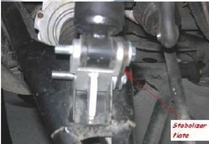
Put the end of the sway bar in line with hole "C" of the sway bar offset plate and slide a 2" bolt through the end of the sway bar and then the stock spacer and finally through hole "C" and put a nut on the end like pictured below.
