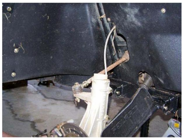
Drop the strut plug into the bottom of the strut cartridge, this is used to space up the actual strut/shock.
