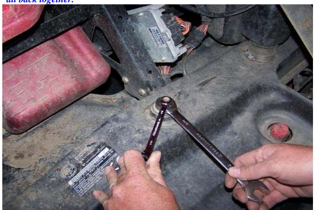
Now loosen the strut from the strut cartridge below, for this, you will need a pair of  $\frac{1}{2}$ " wrenches or sockets or 1 of each, and just loosen the 2 bolts on the aluminum strut
