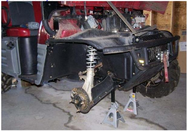
Using a 3/8" wrench or socket, and a 3/4" wrench, loosen the top strut bolt but remember the order in which all of the washers/spacers are placed for when you put it
