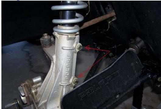
Once loose, reach between the spring coils and slide the lower part of the strut (the cylinder) up the center shaft until it clears the top of the strut cartridge and pull it
